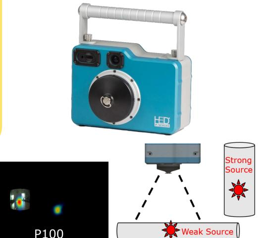
When imaging a weak source in the presence of a strong source, the H100 sees only the strong source, but the P100 can see the weak source because of the P100's collimator.
