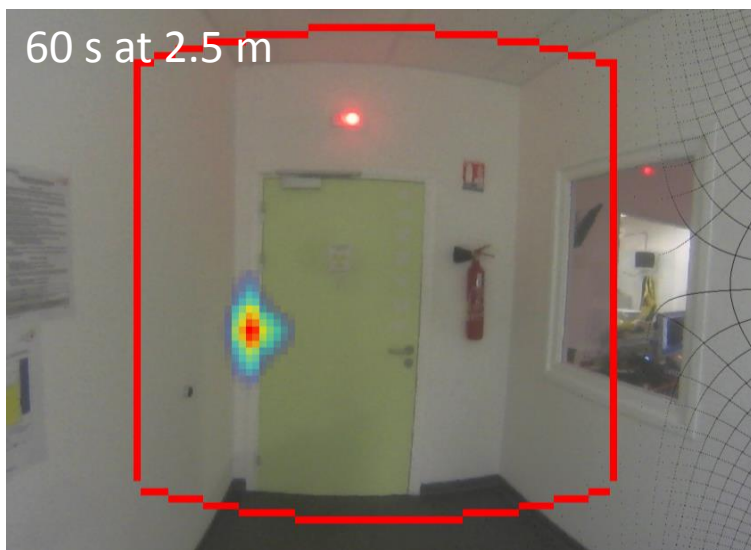
50-100 keV x-ray leakage around door hinges at a hospital
