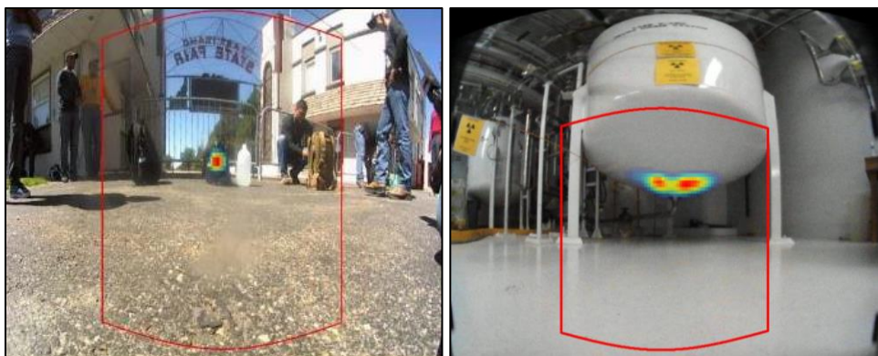
Images of 99m Tc (140 keV) in a backpack and 137 Cs (662 keV) in a water tank using the H Series
